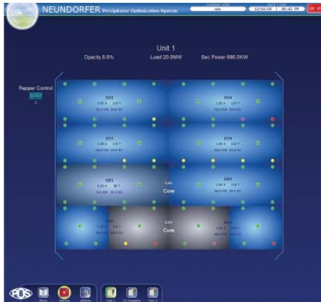
Installation of Neundorfer controls began in January 2010, and was completed by the summer. A Neundorfer technician visited ecomaine, installed three of the 12 power controls, and showed technicians how to put in the new units so they could finish the job on their own. Change-out of the controls was done creatively to minimize downtime. For example, one of the units was installed during a single-day furnace maintenance outage.
