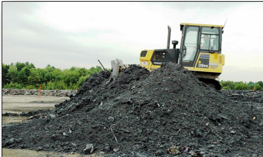
Ash from the waste-to-energy is trucked just 3 miles to the ashfill. Bulldozers level the ash after each delivery.
